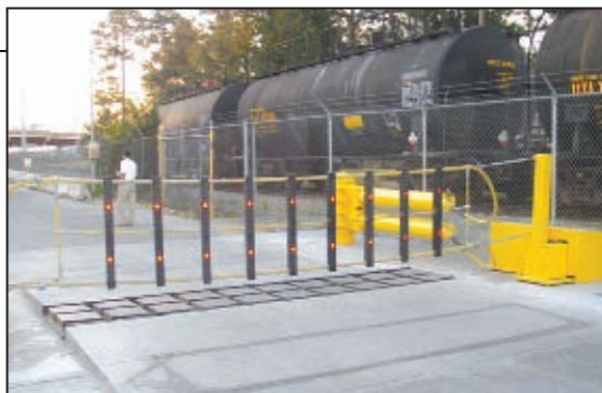
FIGURE 2. Ground retractable automobile barriers (GRAB) stop the unauthorized entry of vehicles up to 15,000 lb, traveling at speeds up to 50 miles per hour
