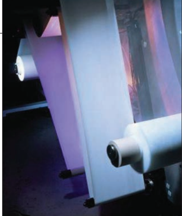
FIGURE 4. Quality control is applied during membrane fabrication. Here a membrane sheet is being rolled on the manufacturing floor
